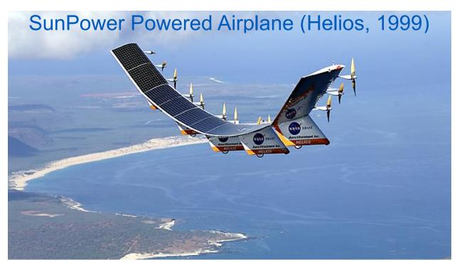
The NASA Helios airplane had 14 electric motors that used SunPower all-black high-efficiency cells to take off and land on its own power. In 2001, it set an all-time altitude record of 96,863 feet, which still stands. The F-15 Eagle, a mach 2.5 fighter, capable of accelerating while climbing vertically, has a service ceiling of 72,000 feet.
